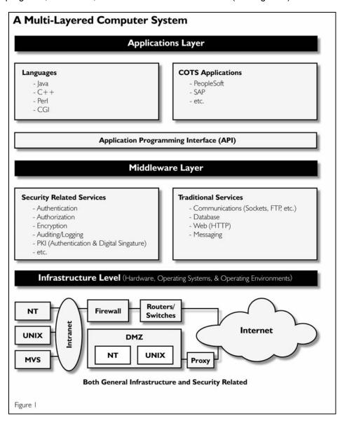
Figure 1: A Multi-Layered Computer System
